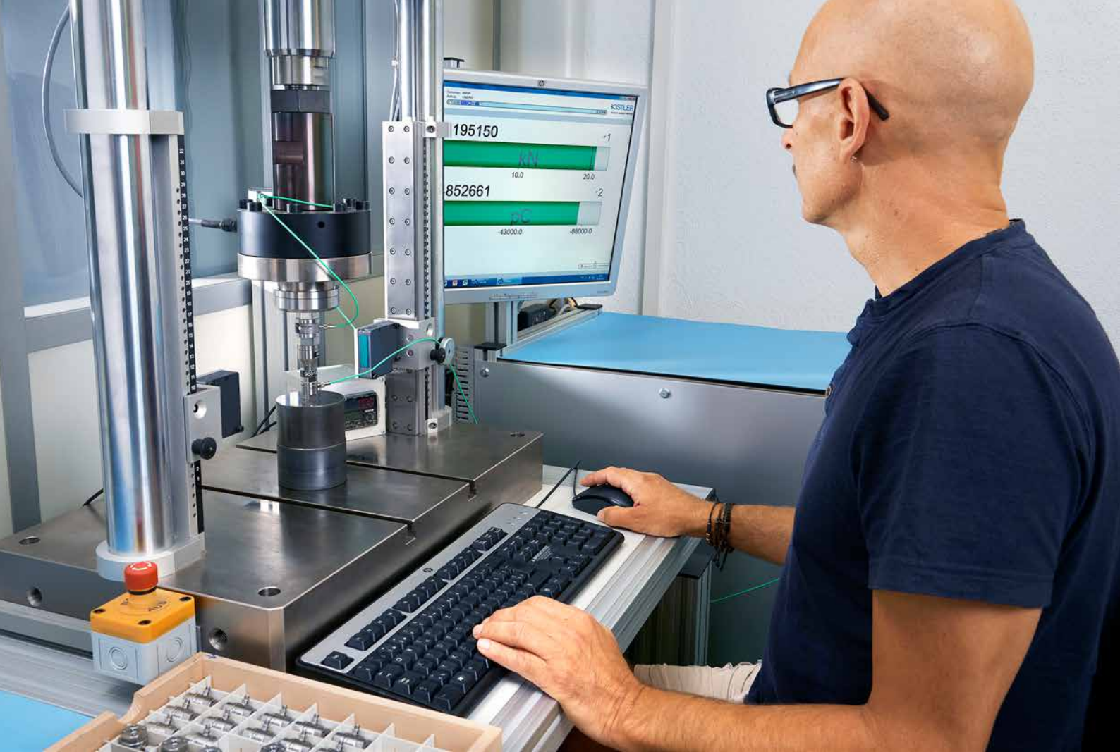
Sensors must be meticulously calibrated in order to guarantee reliable measurement results
