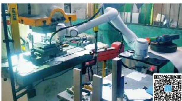
08 Loading and unloading materials for stamping machine
